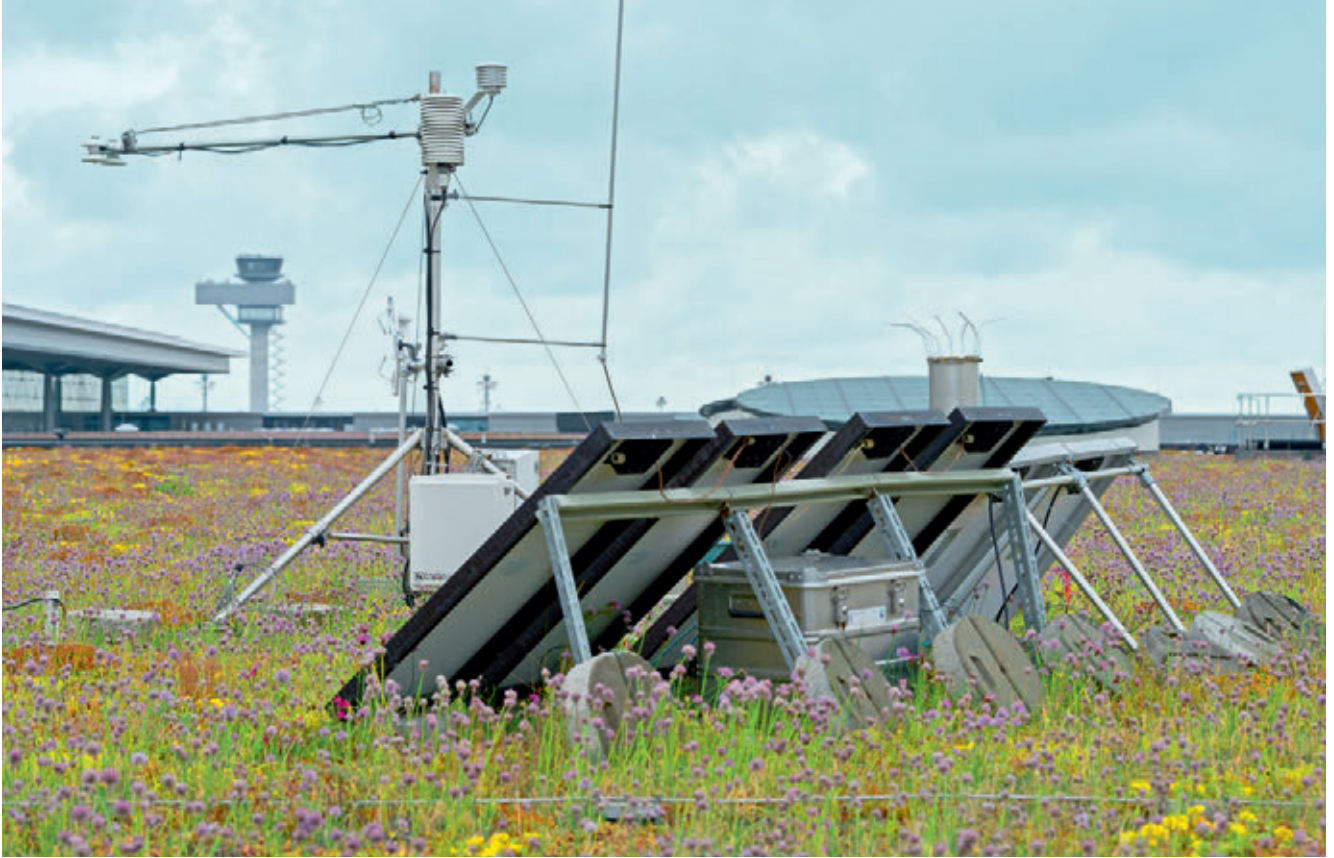
Researchers of the Technical University of Braunschweig examined based on the example of the planted multi-storey car park roofs of the BER, which contribution the green roofs make to improving the city climate in 2016.
