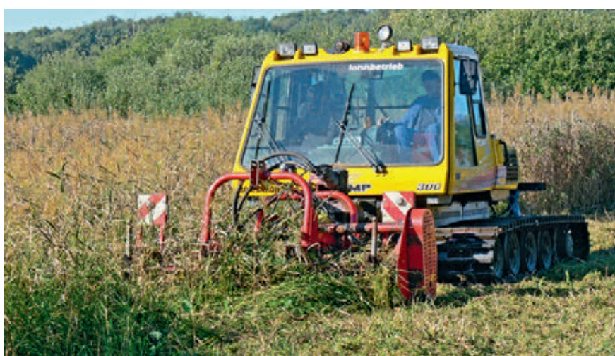
Special caterpillar with haulm cutter for the reactivation of wet meadows
